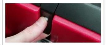
Disconnect the battery by sliding back the silver slider [this is part of the connector] and turning the connector anti-clockwise. 4. As advised by the airline; close the cover and replace the seat to transport Wizzybug whole, or remove the battery to carry on board.
